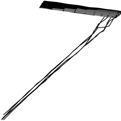
Fig. 6 Streamlines from PMARC-12 for the baseline wing.
